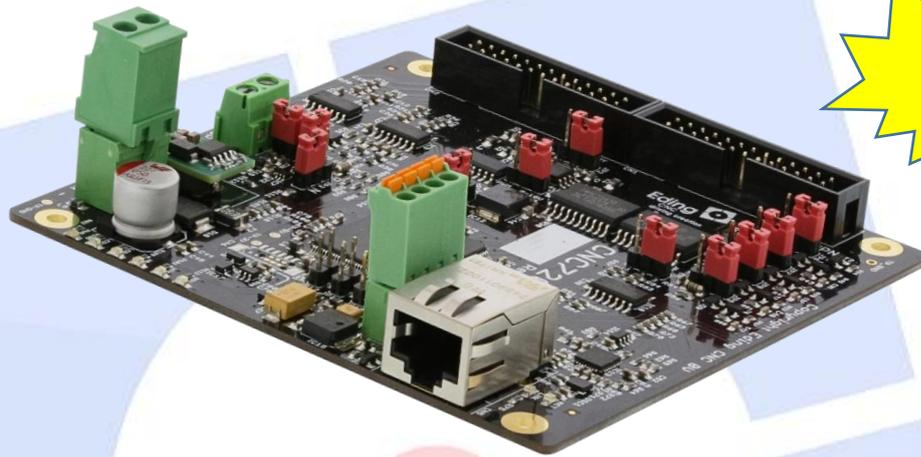
This CNC controller is the second of a new generation of Eding CNC controllers. Besides a standard 100Mbit Ethernet interface, the step frequency increased to 400 kHz.
